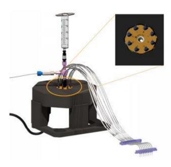
Connect the pump, from its output port to either the centre of the MultiFlow8 or to the 3-way adapter, depending on the Multiflow8 setup. With all valves open, run the 'dispense reagents' step several times to wash through all ports of the MultiFlow8.
